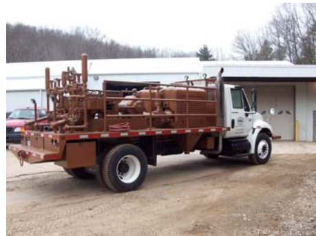
CSi's Cement Pumping Unit
